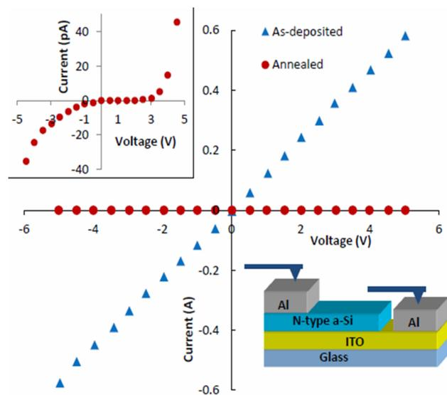
**Figure 5.** Current-voltage characteristics of ITO/n-type a-Si:H thin film junctions after deposition and annealing. The as-deposited n-type Si film shows ohmic contact with ITO. After annealing, the contact deteriorates to a Schottky type contact with increased contact resistance. The top inset shows the current-voltage characteristics of the annealed sample. The bottom inset shows the schematic of the sample used for the measurement.
