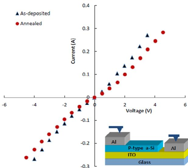
**Figure 4.** Current-voltage characteristics of ITO/p-type a-Si:H thin film junctions after deposition and annealing. The inset shows the schematic of the sample used for the measurement. The nearly linear current-voltage curve indicates the formation of ohmic contact between ITO and p-type silicon.
