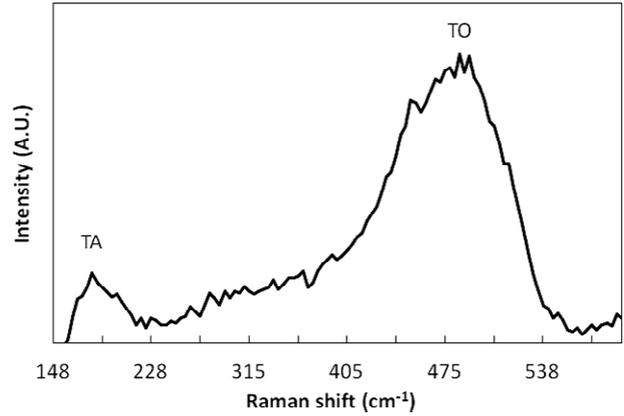
**Figure 2.** Raman spectroscopy scan of as-deposited p-type a-Si:H film. The peaks at  $160$  and  $480\text{ cm}^{-1}$  correspond to amorphous Si-Si transverse acoustic (TA) and transverse optic (TO) vibrational modes, respectively.
